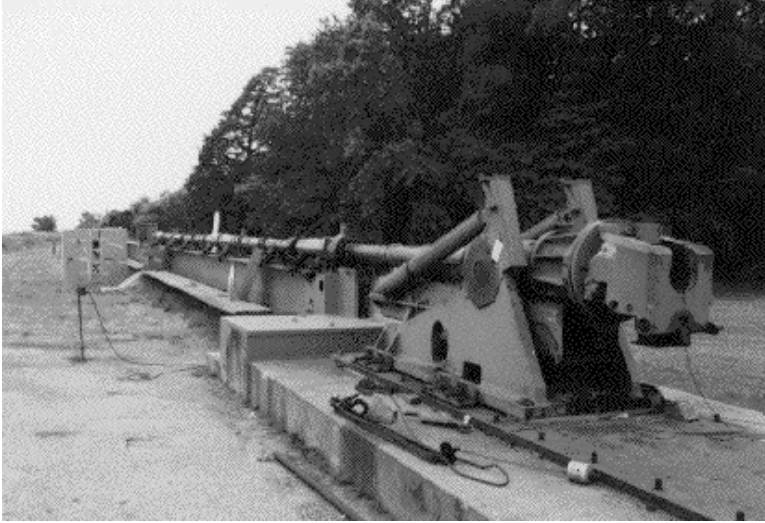
Figure 14 Closeup of the 120mm cannon injector to ram accelerator barrel.
