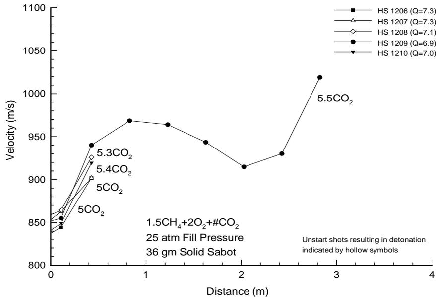
Fig. 14. Velocity versus distance data for 850 m/s entrance velocity with 36 gm solid sabot.
