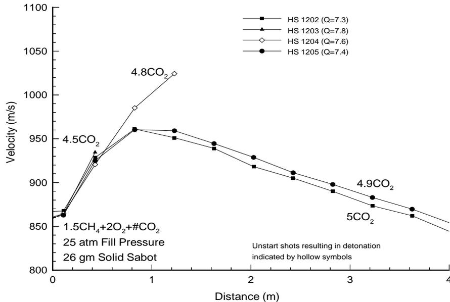
Fig. 13. Velocity versus distance data for 850 m/s entrance velocity with 26 gm solid sabot.
