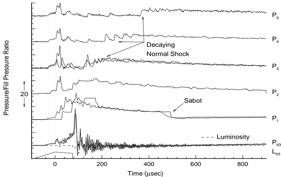
Fig. 15. Tube wall pressure and luminosity traces for HS1205.
