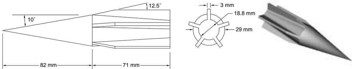
Fig. 4. Standard ram accelerator projectile.
