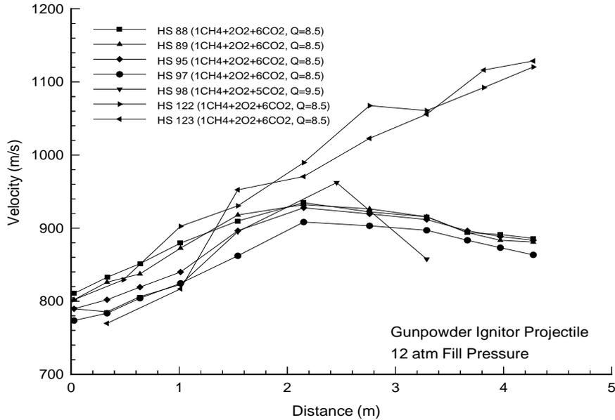
Fig. 7. Velocity versus distance data for early low entrance velocity shots.
