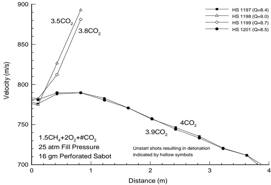
Fig. 11. Velocity versus distance data; 780 m/s entrance velocity with 16 gm perforated sabot.
