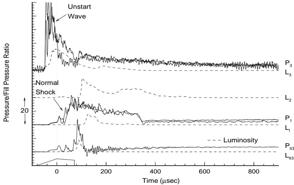
Fig. 16. Tube wall pressure and luminosity traces from HS1191.
