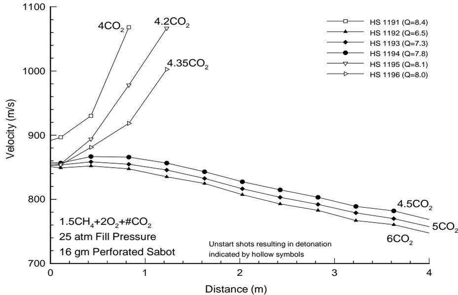
Fig. 12. Velocity versus distance data; 850 m/s entrance velocity with 16 gm perforated sabot.
