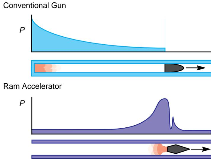
Fig. 2. Pressure profiles of a conventional gun and a ram accelerator.
