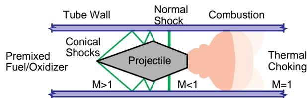
Fig. 1. Ram accelerator subdetonative mode of propulsion.
