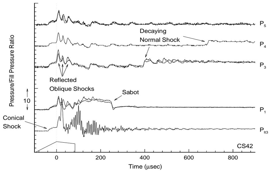
Fig. 10. Tube wall pressure traces for shot into non-reactive mixture.
