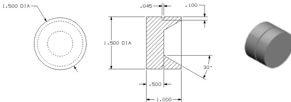
Fig. 8. Solid sabot with a Bridgman seal.
