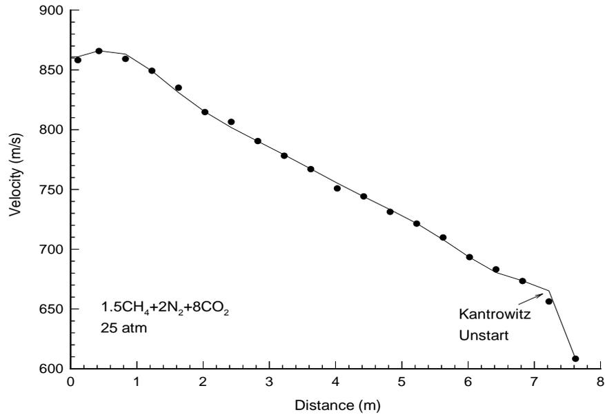
Fig. 9. Velocity versus distance data for shot into non-reactive mixture.
