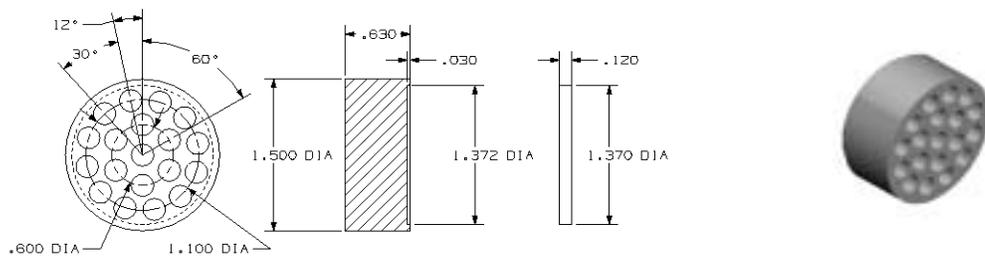
Fig. 5. Standard perforated sabot.
