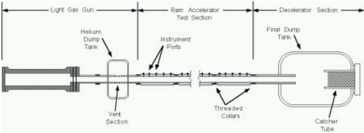
Fig. 3. Ram accelerator facility schematic.
