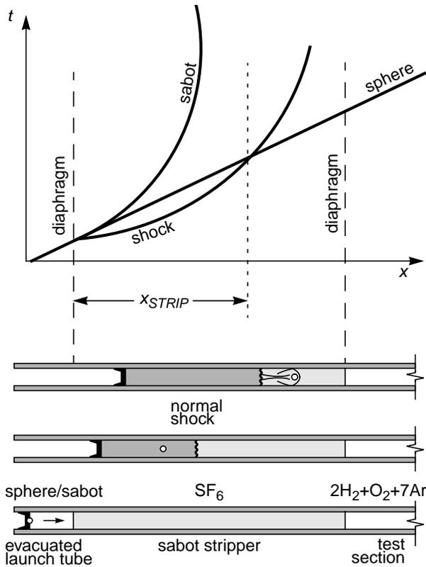
Fig. 3  $x-t$  diagram of the sabot stripping process.
