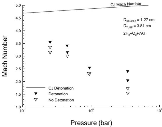
Fig. 5 Results from firing spheres into a small diameter detonation tube.
