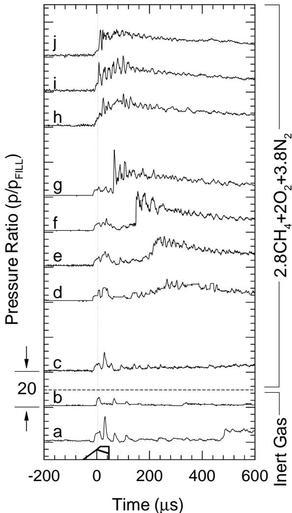
Fig. 9 Pressure data from ram accelerator experiment with combustion wave stripping. Note ignition in wake.
