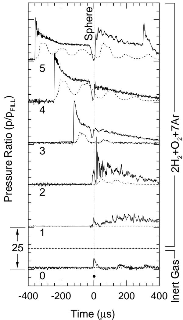
Fig. 4b Pressure (solid line) and luminosity (dashed line) data for a sphere traveling at 1100 m/s (65% CJ speed).
