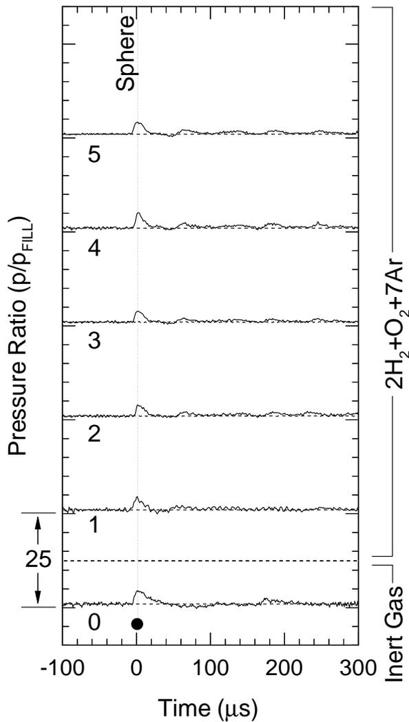
Fig. 4a Pressure (solid line) and luminosity (dashed line) data for a sphere traveling at 800 m/s (47% CJ speed).
