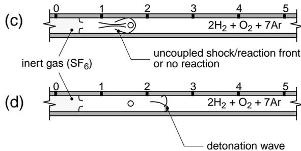
Fig. 1 Schematic of detonation initiation by blunt projectiles:
