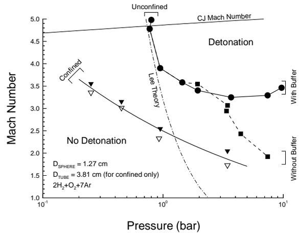
Fig. 6 Comparison of detonation by projectiles in confined and unconfined experiments.
