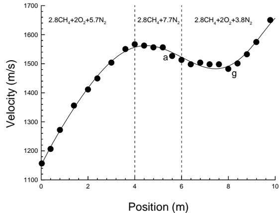
Fig. 10 Velocity–distance data for the combustion stripping experiment.
