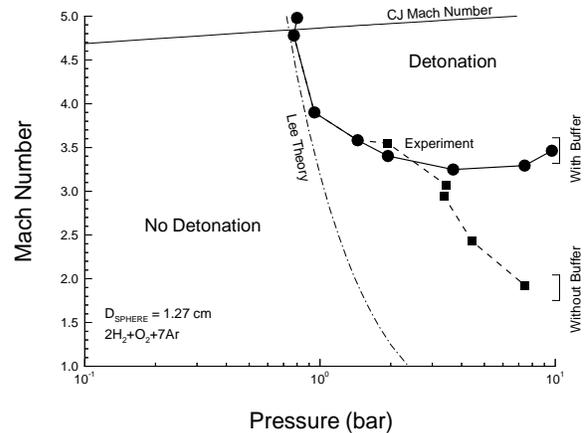
Fig. 2 Results from firing spheres into a large diameter detonation chamber.
